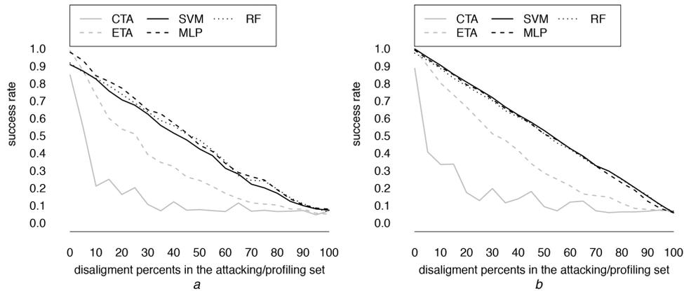
**Fig. 4** Probability to retrieve the target value as a function of the number of misalignments in profiling and attacking sets for CTA, ETA, SVM, MLP, and RF based on the DPA Contest V4.2
