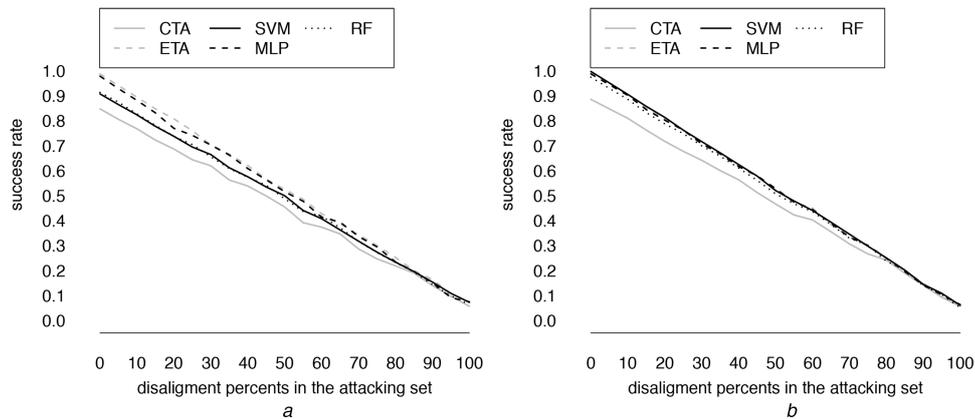
**Fig. 3** Probability to retrieve the target value as a function of the number of misalignments in attacking set for CTA, ETA, SVM, MLP, and RF based on the DPA Contest V4.2
