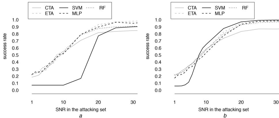
**Fig. 6** Probability to retrieve the target value as a function of the SNR (in dB) in attacking set for CTA, ETA, SVM, MLP, and RF based on the DPA Contest V4.2
