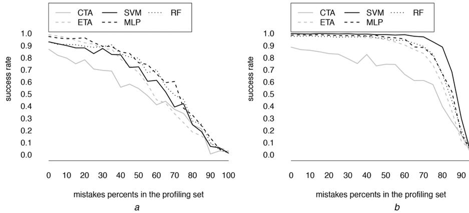
**Fig. 1** Probability to retrieve the target value as a function of the number of mistakes in profiling set for CTA, ETA, SVM, MLP, and RF based on the DPA Contest V4.2
