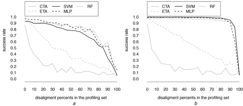
**Fig. 2** Probability to retrieve the target value as a function of the number of misalignments in profiling set for CTA, ETA, SVM, MLP, and RF based on the DPA Contest V4.2
