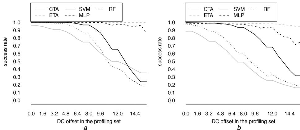
**Fig. 7** Probability to retrieve the target value as a function of the DC offset applied on the leakages from the profiling set for CTA, ETA, SVM, MLP, and RF based on the DPA Contest V4.2
